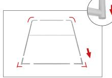
**Step 5:** Assemble post (75) into base plate or optional feet with screw by hand turning post and tightening into place.
